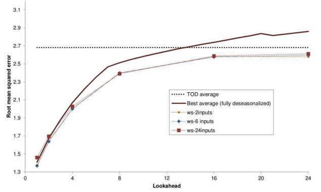
**Figure 2: Forecasting accuracy of evolved ANNs using only wind speed input data.**
